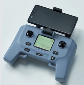
One standard controller and ACSL's Remote ID module are standard equipment.
